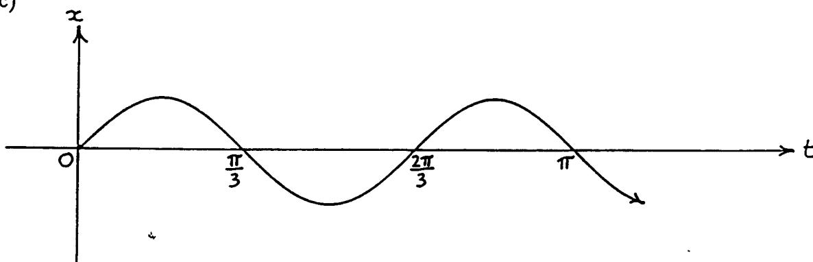
The diagram shows the displacement  $x$  cm from the origin at time  $t$  seconds of a particle moving in simple harmonic motion.
