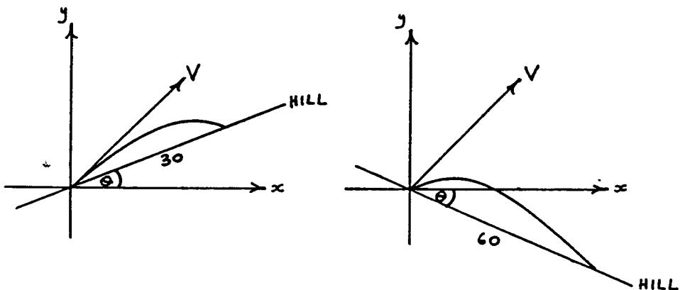
The man is now standing on a hill inclined at an angle  $\theta$  to the horizontal. He throws the ball at the same angle of  $45^\circ$  to the horizontal and at the same speed of  $V$  m/s. If he can throw the ball 60 m down the hill but only 30 m up the hill, use the result in part (ii) to show that:
